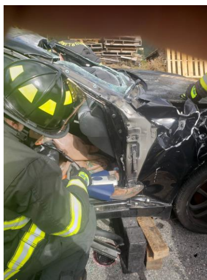
Firefighters using Res Q Jack's to stabilize a vehicle and performing extrication.
